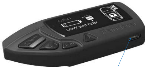
Micro-USB port for charging and software updates
