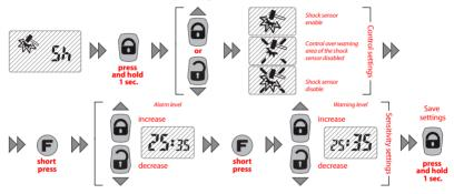
For prompt remote adjustment of alarm and warning levels of the shock sensor enter the settings menu, select from with button presses and press button for 1 second. Press button to cycle between control and sensitivity settings of warning and alarm sensor levels.
