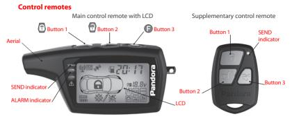
Two-way remote is the main mean of control over the system. For easily distinguishable notifications the remote uses 16 ringtones. Each ringtone matches particular event.
