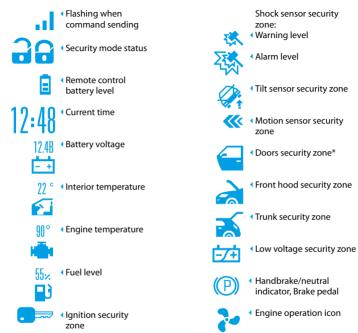
\* Separate display indication of doors, original alarm status, fuel level depend on information in CAN-bus digital protocol of specific car
