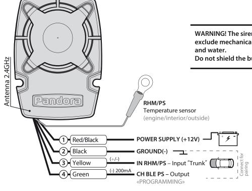
WARNING! The siren must be installed in the places that exclude mechanical damage and ingress of corrosive liquids
