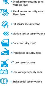
\*Separate display indication of doors, factory alarm status, engine temperature depends on the information in CAN-bus digital protocol of specific car. Fuel level indication depends on the information in CAN-bus digital protocol, or on the fuel level sensor analog output signal (require additional connection).
