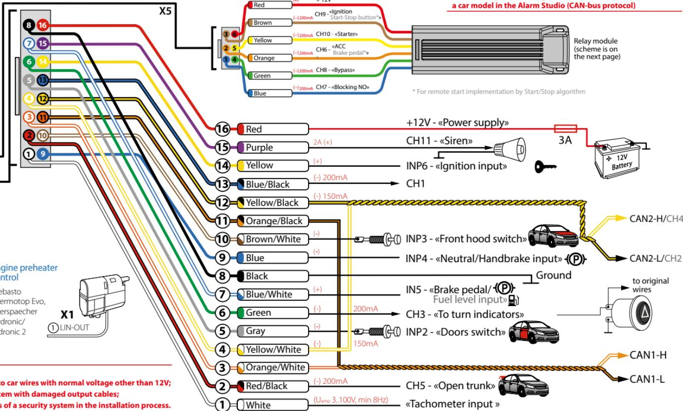
**WARNING! Before starting the installation of the system, select a car model in the Alarm Studio (CAN-bus protocol)**
